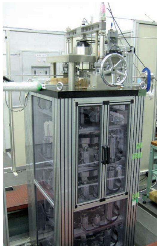
Figure 1 External appearance of controlled-clearance pressure balance in NMIJ
