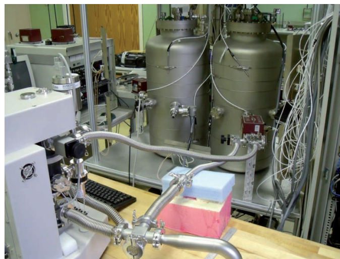
Figure 2. Digital piston cylinder connected to the static expansion system SES by a differential pressure transducer CDG.
